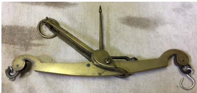
96 Oogjesbalans, Becker-Arnhem, messing schaaltes Nagel-1818 [648]
